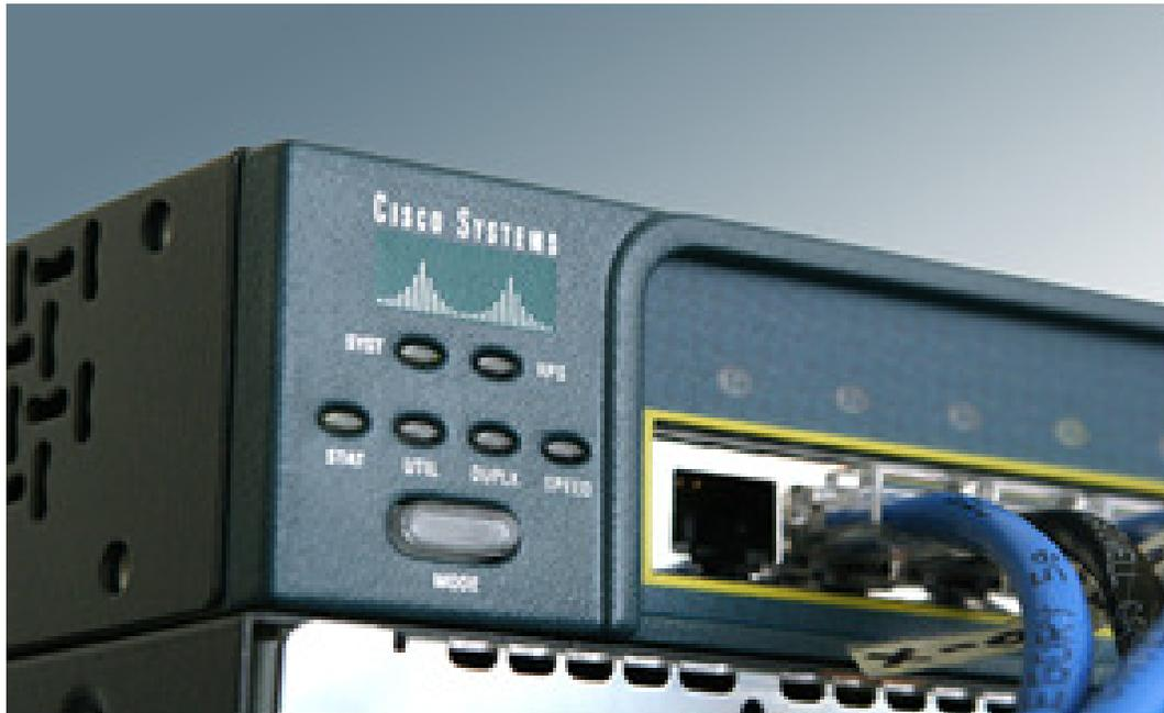
If modem is OK, the first step is to remove the Tulip LAN cable from switch and connect a LAN cable from CISCO 1905 Router GEO/O port to Switch port.
